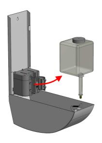
6. Pull silicone tube downwards and place the outlet nozzle in the slot. Make sure that the collar is located under the pump housing.
