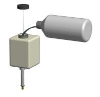
5. Pull silicone tube downwards and place the outlet nozzle in the slot. Make sure that the collar is located under the pump housing.
