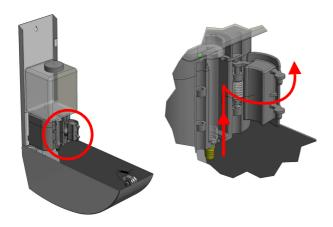
Mount the soap container by gently pushing it into the groove on the pump housing.
